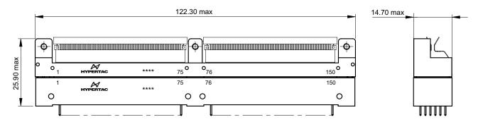
Maximum dimensions of mated connectors equipped with three dielectric inserts
