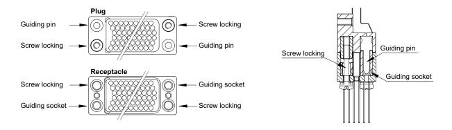
Connector supplied with two coding keys and two screw locking (only connectors without backpanel)
