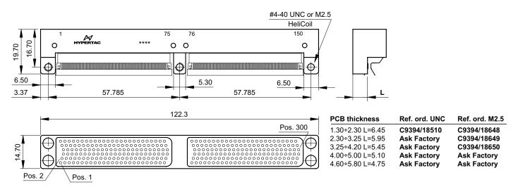
Receptacle connector, 450 socket contacts, surface mount tail terminal style, board package thickness from 1.30 to 5.80
