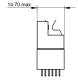
Maximum dimensions of mated connectors equipped with two dielectric inserts
