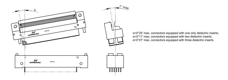
Maximum permissible displacement in orde to ensure the suitable fully insertion of the connector halves
