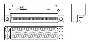
PCB thickness 1.30÷2.30 L=6.45 Ref. ord. Ask Factory PCB thickness 2.30÷3.25 L=5.95 Ref. ord. Ask Factory PCB thickness 3.25÷4.20 L=5.45 Ref. ord. Ask Factory PCB thickness 4.00÷5.00 L=5.10 Ref. ord. Ask Factory PCB thickness 4.60÷5.80 L=4.75 Ref. ord. Ask Factory
