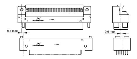
Maximum permissible distance of the connector halves in order to ensure the acceptable electrical engagement made by all contacts
