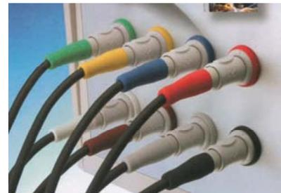
Incorrect mating also can be avoided by using keyed connectors. These incorporate a mechanism that physically prevents the plug and receptacle from being mated if they are an unmatched pair.
